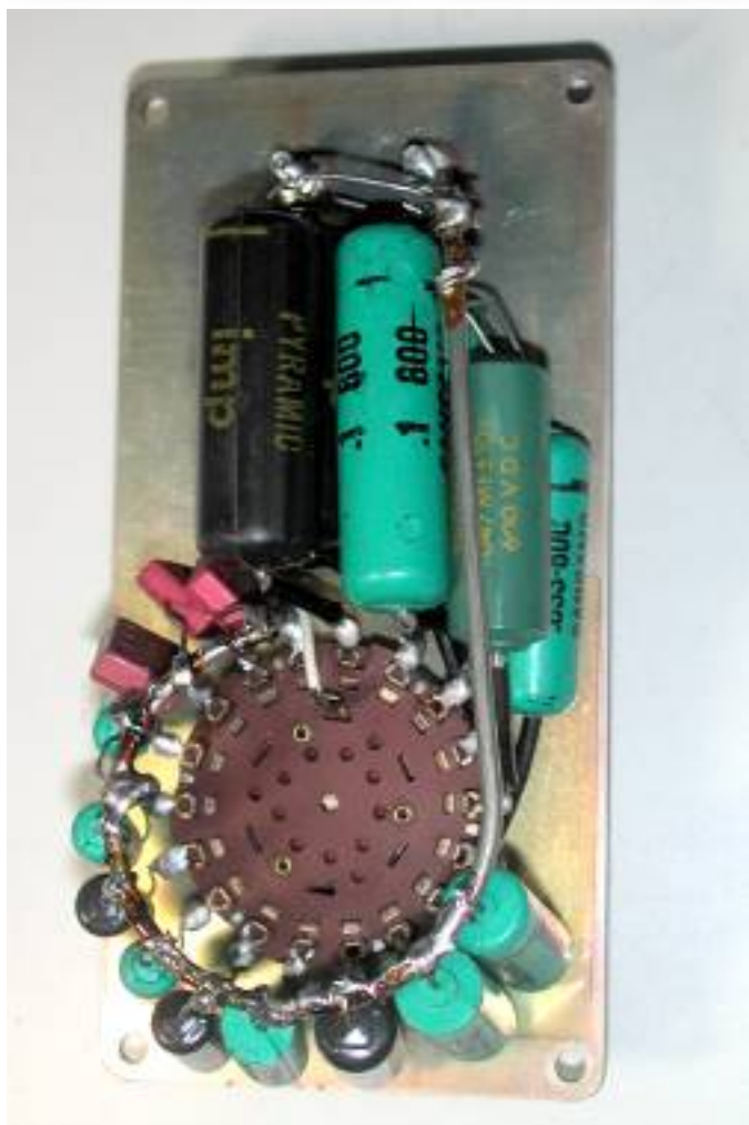
Figure 3: Internal view of the original CS-1.
