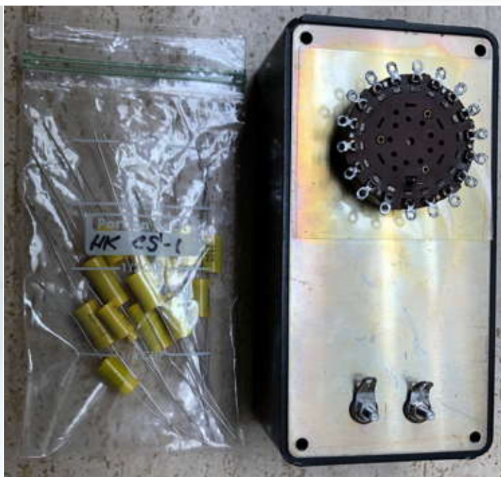
Figure 4: partial reassembled CS-1 awaiting capacitor installation
